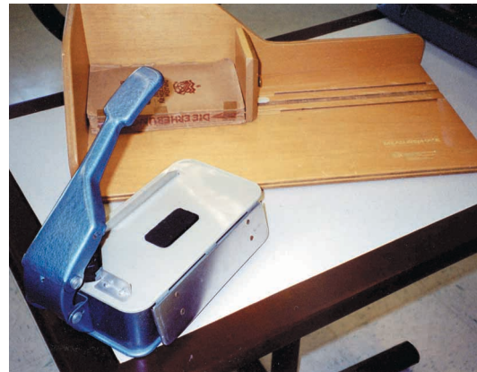
Figure 2. The MEASUREpHASE™ gives quick, accurate book measurements and the Corner Rounder improves the appearance of the final product.
