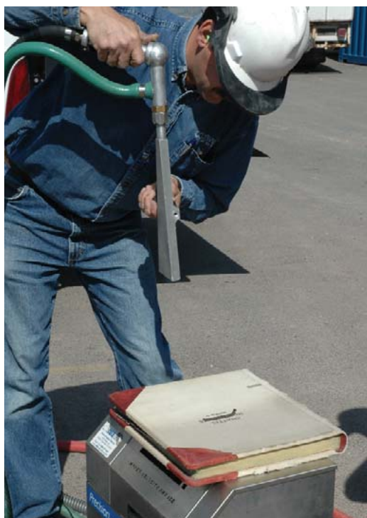
Randell Heath, President, CO 2 LDSWEEP Dry Ice Blasting, at work removing soot from a Sevier County record book. Photo credit: Randy Silverman
