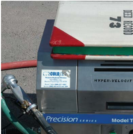
Second test sample; cleaning results from a lightly soot damaged 20th century record book covered in a protective white canvas jacket. The area of the jacket left of the number “73” and below the word “Deed” was wiped with a natural rubber sponge; right of the number “73” and below the word “Deed” was vacuumed with a HEPA vac; and, the area above the words “Deed Record” was dry ice blasted. Photo credit: Randy Silverman
