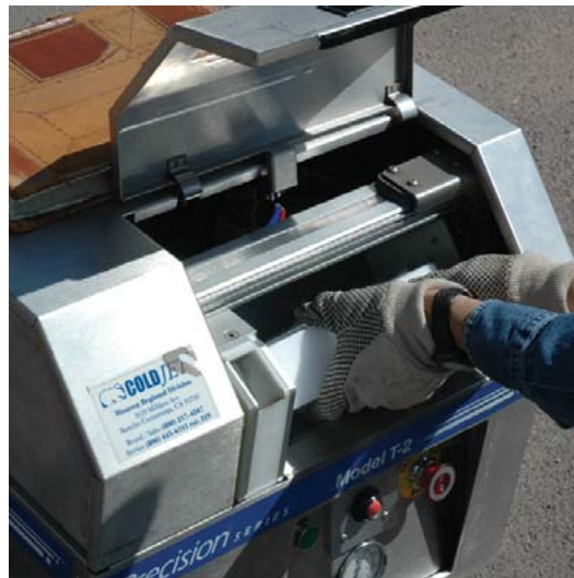
An 18th century full-leather record book sitting on the Alpheus Precision Series™ Model T-2 dry ice blasting machine as it is refilled with block dry ice. Photo credit: Randy Silverman
