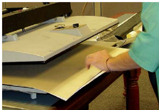
Figure 9. When the press reaches 175°F, the folder containing the photographs is placed in the pre-heated press.
