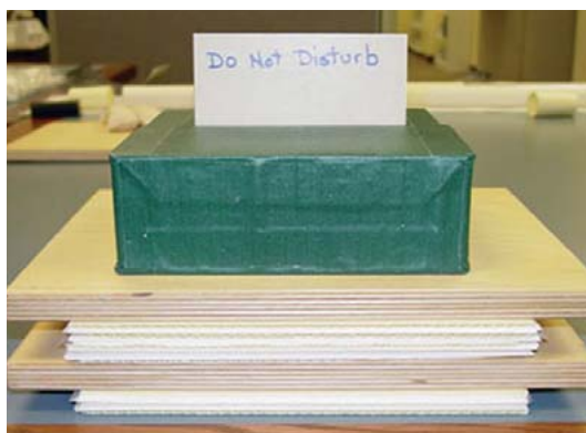
Figure 10. After the photographs have been layered in the drying stack, weight is applied to the top and the stack is allowed to sit undisturbed for several hours.
