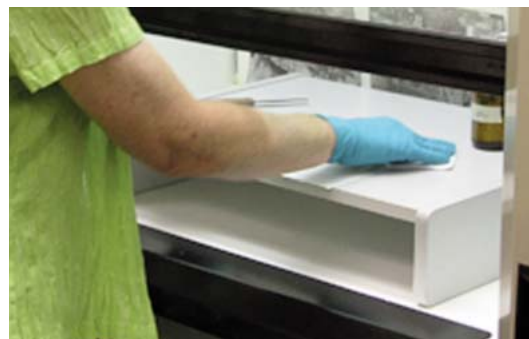
Figure 4. Disposable nitrile gloves are worn and the work is completed under a fume hood.
