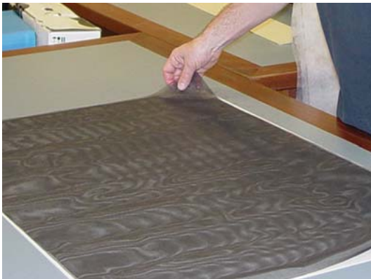
Figure 6. The bottom half of the stack is constructed using a piece of blotter paper dampened with de-ionized water.
