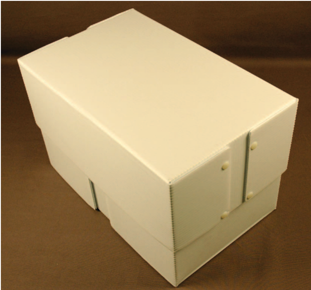
Figure 6: Completed two-piece Coroplast box for an oversized ledger book showing nylon snap rivets used to mechanically fasten the walls of the lid. (Photo credit: Hunt)
